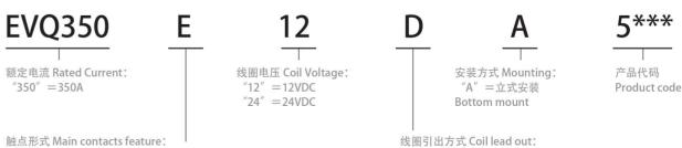
"E" =主触头为一组常开,触头不分极性; 1 form A(ON), non-polarized; "G" =主触头为一组常开, 触头不分极性, 带一组常开辅助触点; 1 form A(ON) add AUX contacts(ON), non-polarized;
